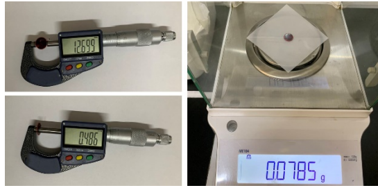
Figure S19 The SC4Q pellet obtained by powder pressing method under 11 MPa.
