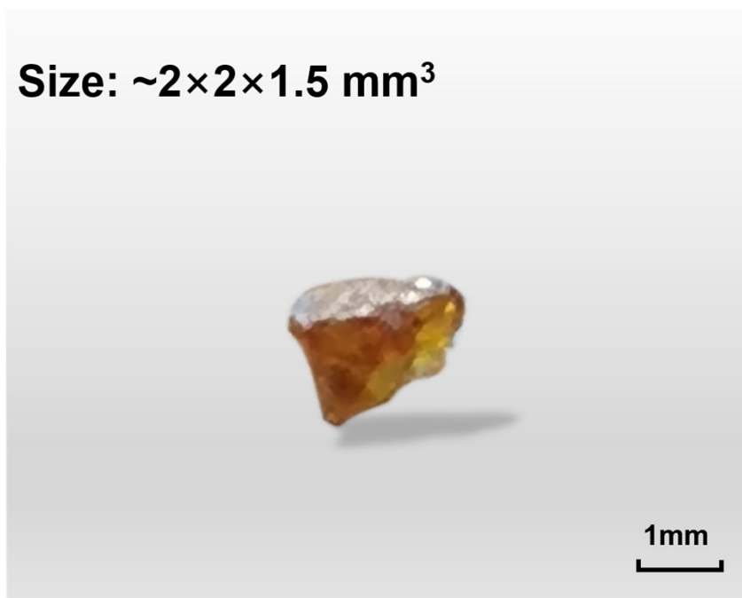
Figure S2. The as-grown single crystal of LVTO.
