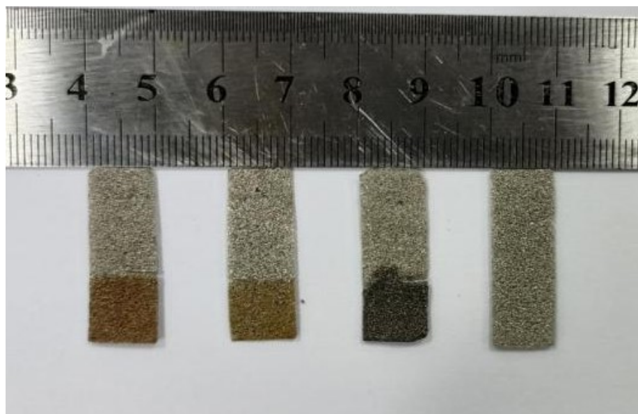
Fig. S3 V_2O_5 -FeOOH, FeOOH, and IrO_2 ink-loaded electrodes and Ni foam (From left to right).
