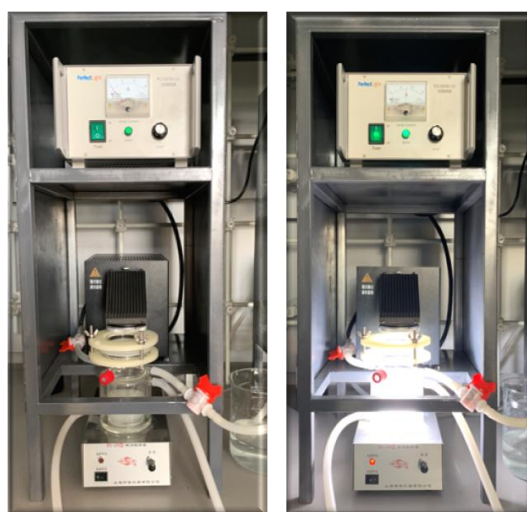
Figure S10. The photograph of the reactor setup for hydrogen evolution experiments. Left is under off light; right is under irradiation by 300 W Xenon light (AM 1.5G) under stirring. The photos show excellent dispersibility of Ni-MOLs in water/MeOH mixture.
