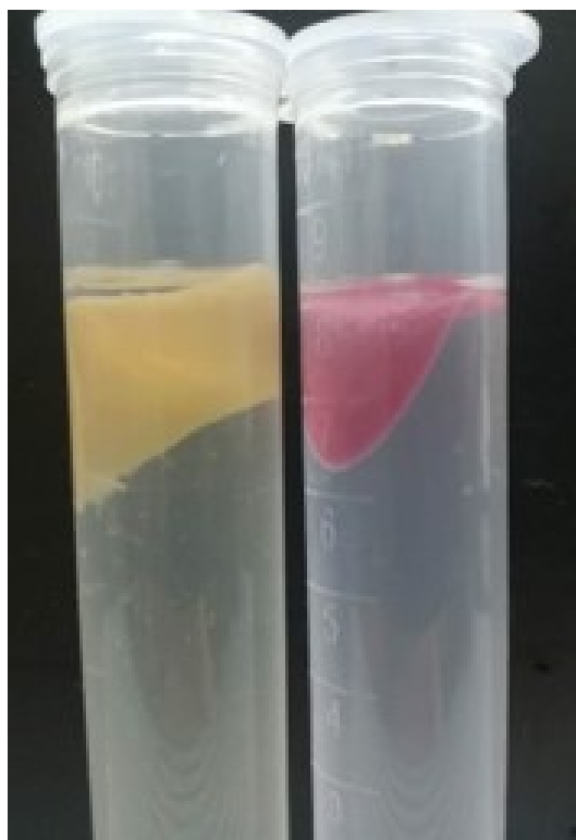
Figure S15. The stability of the catalyst at the gas-water interface. Left (0h), right (24h). The catalyst is easy to oxidize and grow up in the air, which is fatal to the reaction. This system has high advantages because it avoids the oxidation deactivation of catalyst caused by traditional centrifugal drying process.
