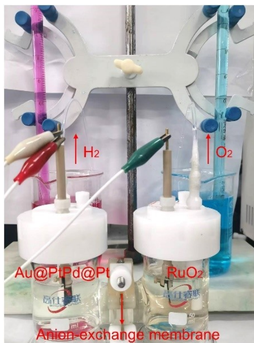
Fig. S19 Digital photograph of the water-splitting electrolyzer and corresponding gas-collecting device.
