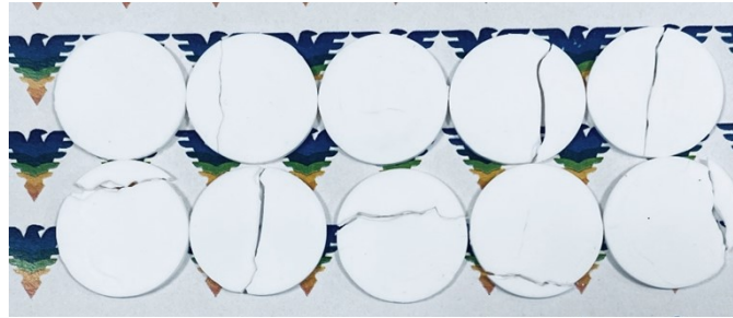
Fig. S5. Photograph for the brown parts, demonstrating the presence of large cracks after thermal debinding. The green parts were thermally debound directly without water debinding.
