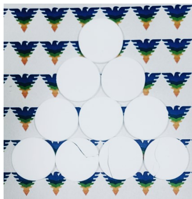
Fig. S7. Photograph for the brown parts, indicating the presence of cracks after thermal debinding. The green parts were processed by water debinding for 1 h then by thermal debinding.
