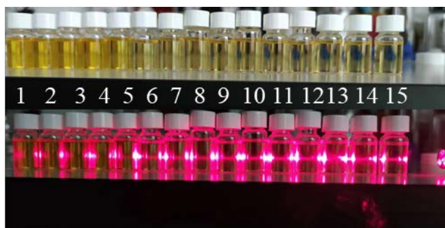
Figure S27. Photos showing the Tyndall effects of 2 in THF solutions upon increasing water content from 0 (THF:H 2 O, 100:0, v/v) to 56 % (THF:H 2 O, 44:56, v/v) in the concentration range of 10 -5 M. (Number 1: 100% THF, 2: 90% THF, 3: 80% THF, 4: 70% THF, 5: 60% THF, 6: 52% THF, 7: 51.5% THF, 8: 51% THF, 9: 50.5% THF, 10: 50% THF, 11: 49.5% THF, 12: 49% THF, 13: 48.8% THF, 14: 48% THF, 15: 44% THF.)
