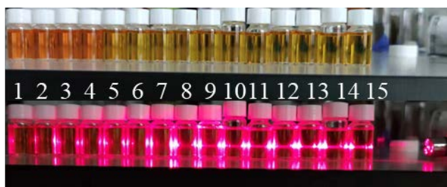
Figure S29. Photos showing the Tyndall effects of 4 in THF solutions upon increasing water content from 0 (THF:H 2 O, 100:0, v/v) to 56 % (THF:H 2 O, 44:56, v/v) in the concentration range of 10 -5 M. (Number 1: 100% THF, 2: 90% THF, 3: 80% THF, 4: 70% THF, 5: 60% THF, 6: 52% THF, 7: 51.5% THF, 8: 51% THF, 9: 50.5% THF, 10: 50% THF, 11: 49.5% THF, 12: 49% THF, 13: 48.8% THF, 14: 48% THF, 15: 44% THF.)
