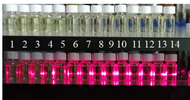
Figure S26. Photos showing the Tyndall effects of 1 in THF solutions upon increasing water content from 0 (THF:H 2 O, 100:0, v/v) to 60 % (THF:H 2 O, 40:60, v/v) in the concentration range of 10 -5 M. (Number 1: 100% THF, 2: 90% THF, 3: 80% THF, 4: 70% THF, 5: 60% THF, 6: 50% THF, 7: 48% THF, 8: 47% THF, 9: 46% THF, 10: 45% THF, 11: 44% THF, 12: 43% THF, 13: 42% THF, 14: 40% THF.)
