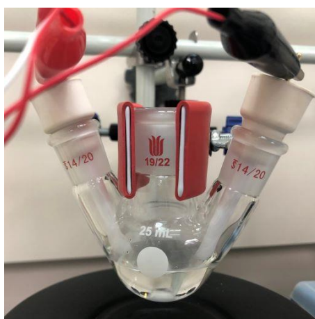
Fig. S1 Setup for the electrochemical iodocyclization with Pt electrodes ( Condition A ).
