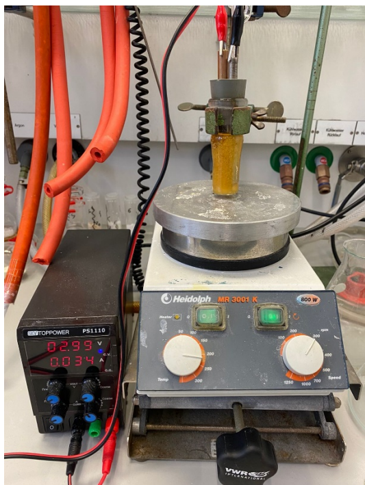
Figure 1. Electrolytic cell and power supply (SKY TOPPOWER PS1110). Electrolytic cell consists of a cylindric glass container (length: 100 mm, diameter: 30 mm), a nickel rod electrode (length: 110 mm, diameter: 8 mm) and a graphite rod electrode (length: 110 mm, diameter: 8 mm) at a distance of 8 mm. The electrodes were suspended 40mm into the solution (equals 11cm 2 of active surface per electrode).
