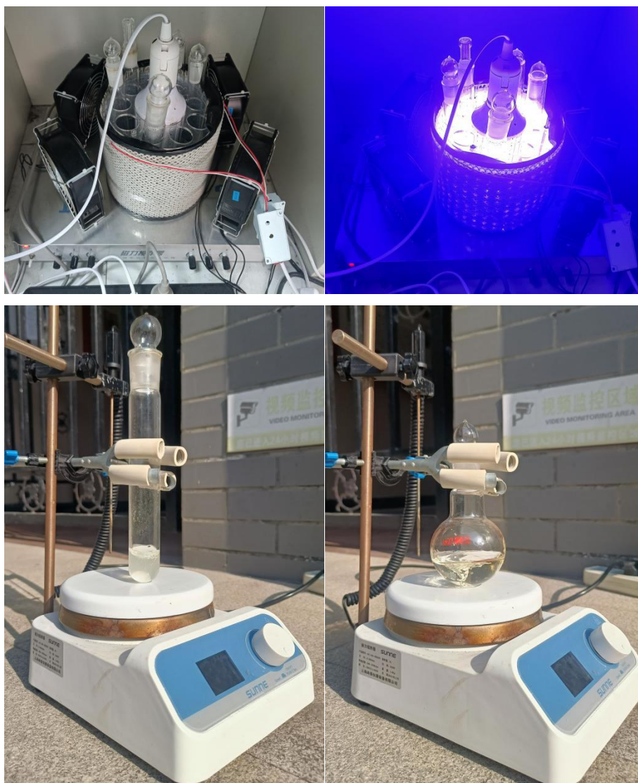
Figure S1. Paralleled photo-reactor at resting state and on work (top); Photo-reaction under sunlight and scale-up experiment under sunlight (bottom).
