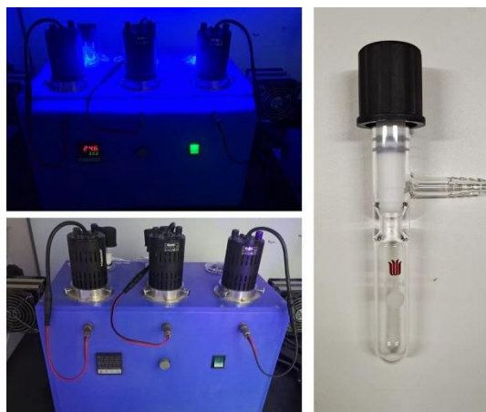
Figure S1 Photo-reaction setup and reaction tube
