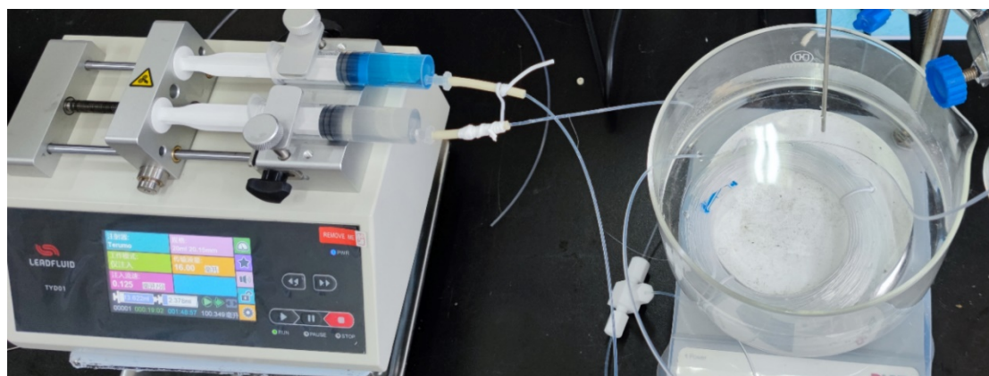
Scheme S2. Details of the micro reactor for the arylated cysteine 3a (0.6 mmol scale)
