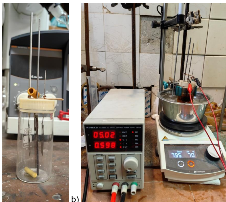
Figure S1. Equipment employed for gram-scale synthesis in the present work a) a sandwich-type cell; b) the model reaction for gram-scale synthesis.
