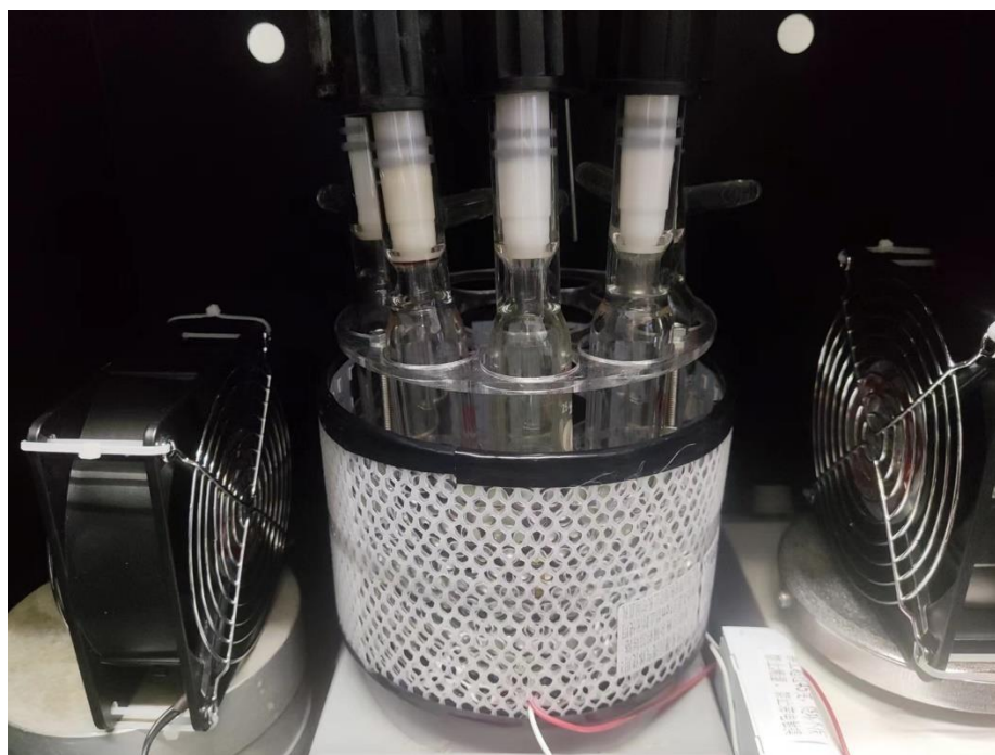
Figure S1-1. Fully assembled 525 nm photoreactor.
