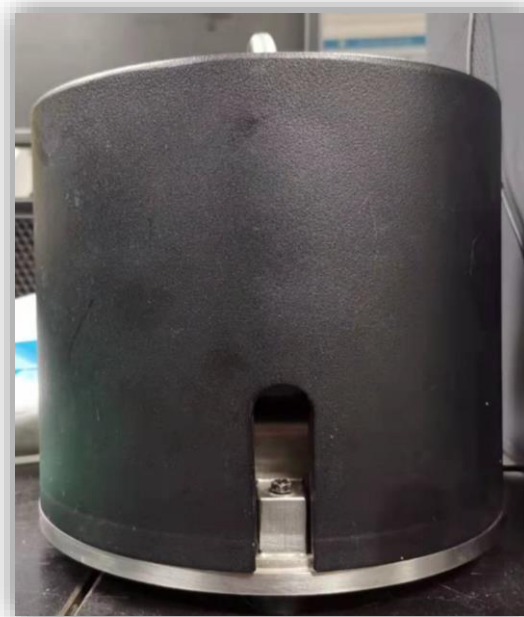
Fig. S1 Schematic diagram of Hotdisk thermal conductivity meter
