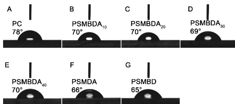
Figure S8 Water contact angle images of pristine PC (A), PSMBDA 10 (B), PSMBDA 20 (C), PSMBDA 30 (D), PSMBDA 40 (E), PSMDA (F), and PSMBD (G) modified PC film.
