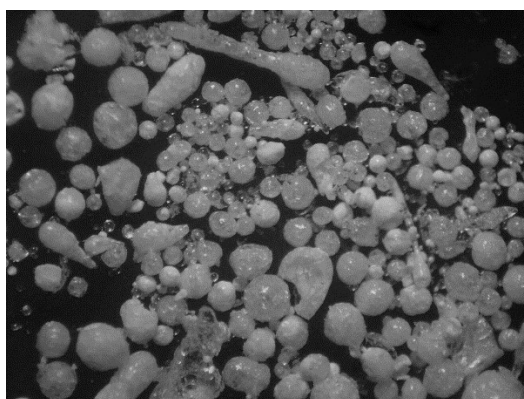
Supplementary Figure S18. Optical microscopy photograph of STH MICROSCAFS® made using 13.7 g of hafnium dichloride oxide octahydrate salt.
