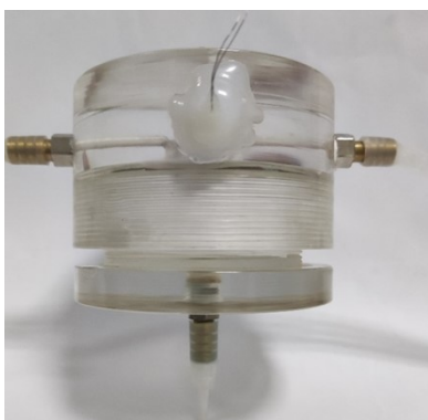
Figure S2. The photo image of the membrane module.
