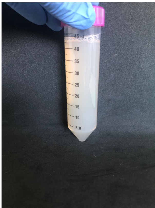
Figure S2: Photograph of CL4 after three months shows no sign of phase separation.
