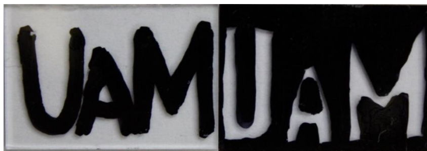
Figure S1. Photograph showing the photomasks used for the photopatterning of a logo of UAM on the ITO glasses.
