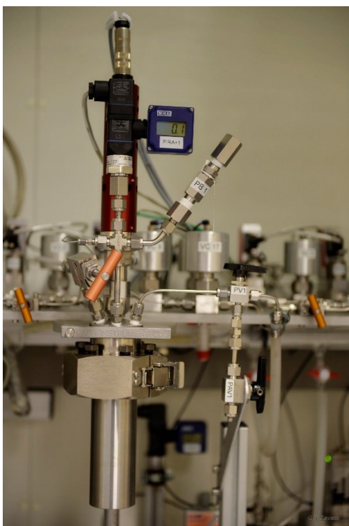
Figure S2: Close up picture of one reactor of the PASCAR plant and the sample loop.
