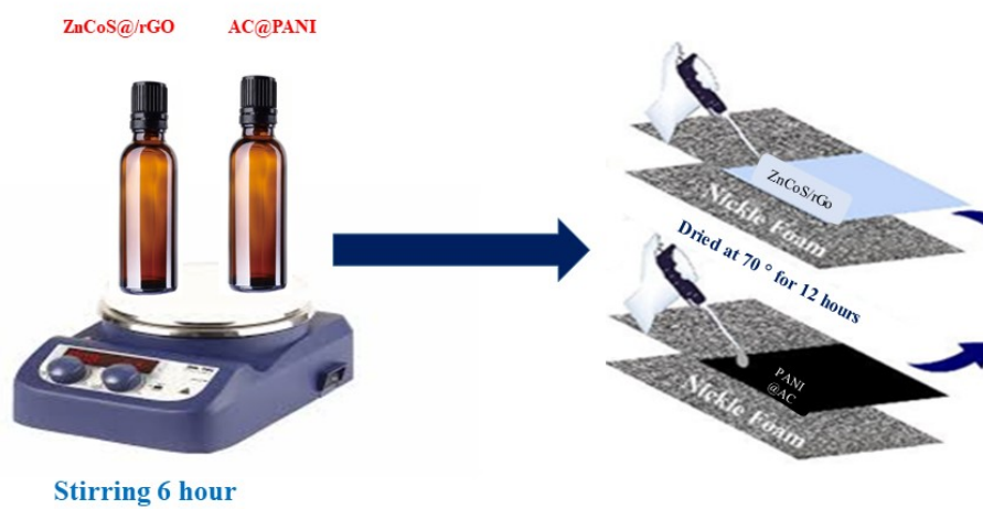
Figure S1: Diagram for preparing electrode for real device.
