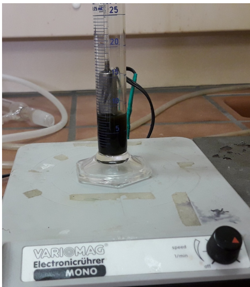
Figure S6. Experimental setup for hydrogenation of IV. The stainless-steel filter is taken out of the solution for visualization.
