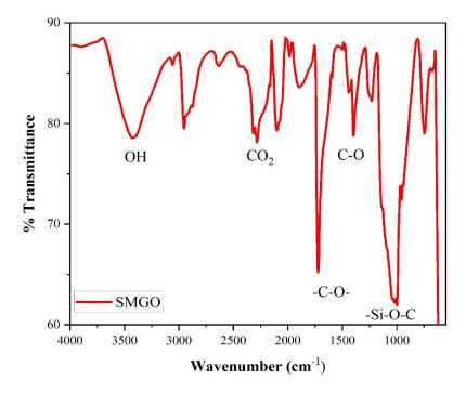
Fig. S1. FTIR spectra of of Silicone-Modified Graphene Oxide (SMGO).
