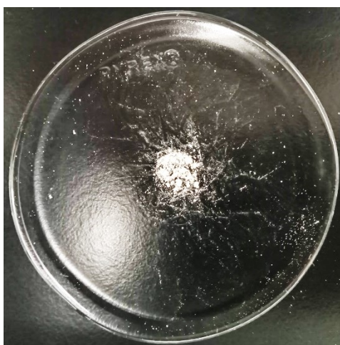
Figure S4: Optical photograph of Ce-carbonate deposited onto \text{TiO}_2 showing white contrast characteristic of \text{Ce}^{3+} and, more specifically, a lack of \text{Ce}^{4+} in the material.
