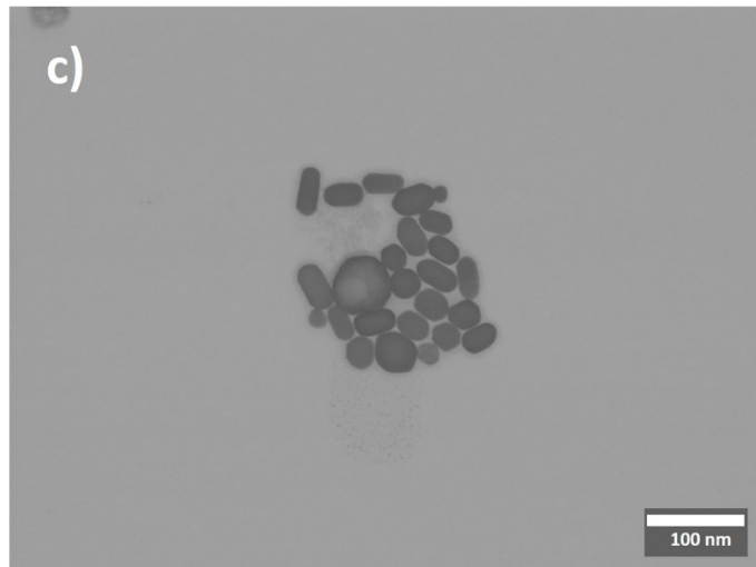
Fig. S3 Gold nanorods (AuNRs) obtained by the seeding method [18]. a) AuNRs suspension; b) absorption spectrum and c) STEM image.
