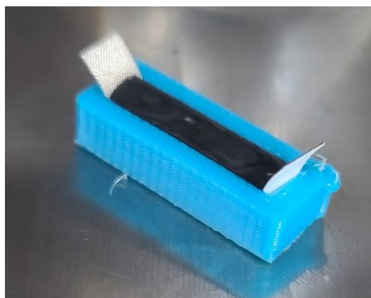
Fig. S1 Digital photo of the sensor made in the 3-D printed mold.
