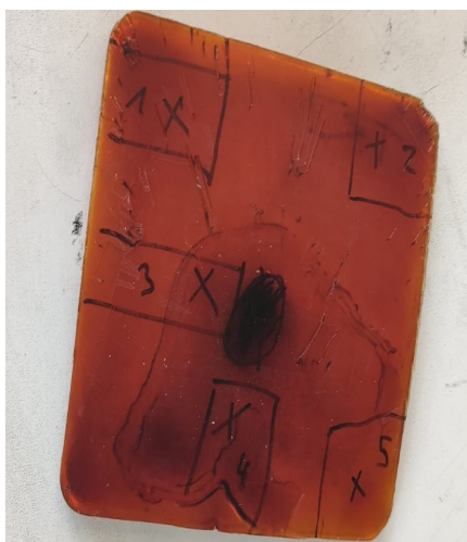
S1 Image of a Limestone-RCFP resin cured in a Teflon mold. The portions on the cured plate from where samples were taken for DSC and FT-IR ATR measurements are labelled.
