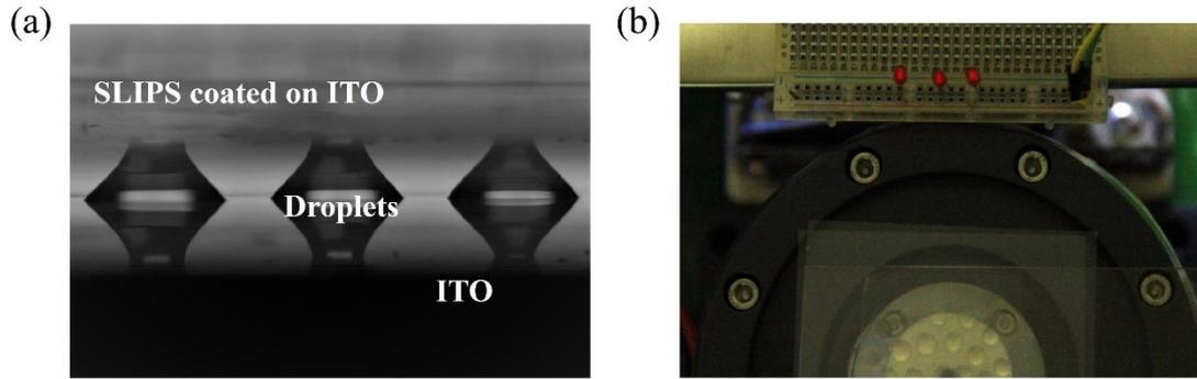
**Figure S4.** Application of REWOD-DEG based on SLIPS. (a) Experimental setup for enhanced power generation, (b) LEDs are lit up using 30 bridges for a sinusoidal input with  $f = 30$  Hz, bias voltage  $V = 200$  V. Total volume of droplets is about  $300 \mu\text{L}$ . The threshold voltage of the red LED is  $1.8$  V.
