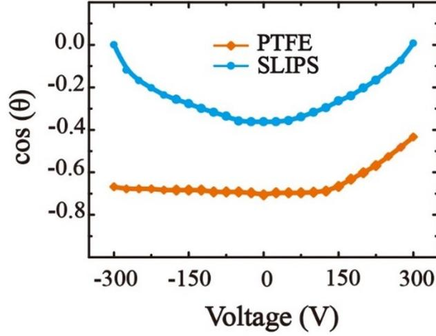
**Figure S2.** Charge trapping test: electrowetting curve of SLIPS and PTFE.
