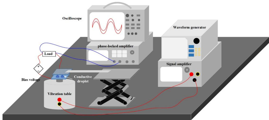
**Figure S7.** Schematic diagram of experimental setup for vibration mechanical energy harvesting based on REWOD-DEG
