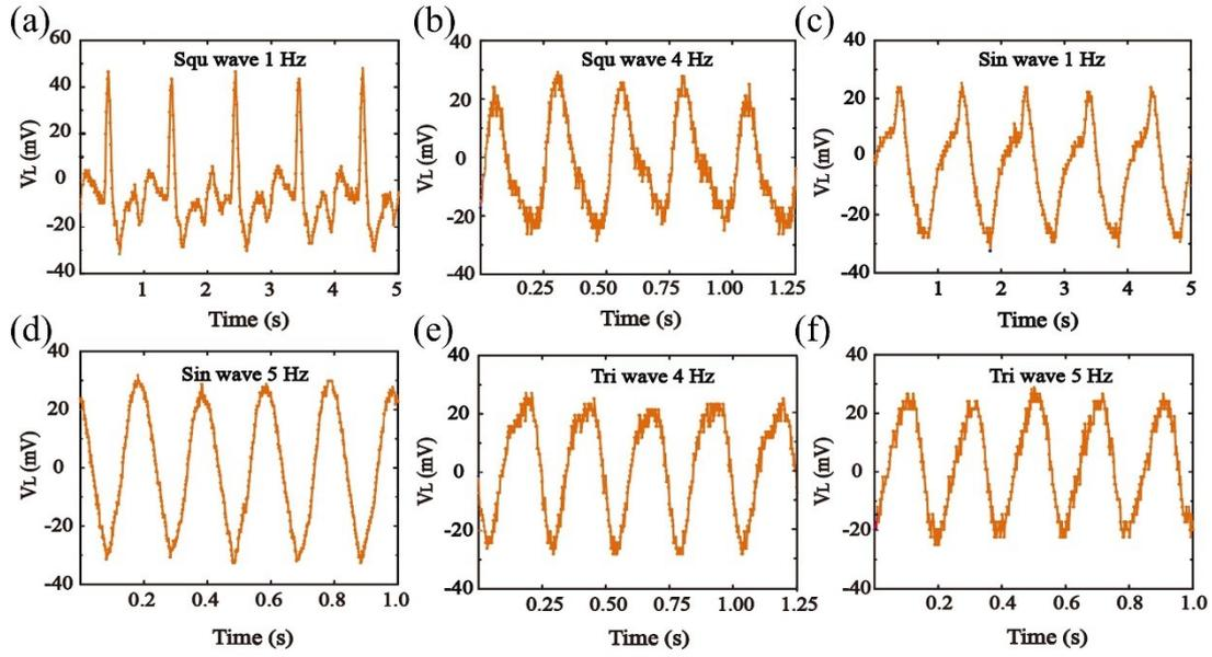
**Figure S3.** The instantaneous voltage output on the load  $V_L$  response to the form (square, sine and triangular) and frequency of the driving waveform applied on vibrator. For all graphs the droplet volume is  $10 \mu\text{L}$  with oscillation amplitude  $L = 1.2 \text{ mm}$ ,  $R_L = 10 \text{ M}\Omega$  and bias voltage  $V = 20 \text{ V}$ .
