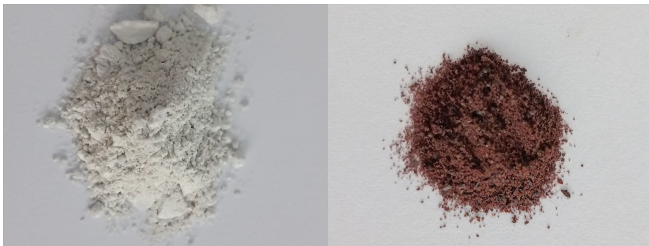
Figure S1: The powder form of Ag-ZnONPs (white) and Ag-ZnONPs@Cy (reddish-brown), respectively
