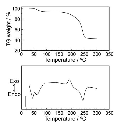
Fig. S1 TG (a) and DTA (b) curves of R=0.95 composite. The TG-DTA measurements were done at the heating rate of 10 °C min<sup>-1</sup> under flowing dry-nitrogen. The scale bar in Fig. S1(b) shows 20  $\mu$ V. Similar results were obtained for triplicate experiments.
