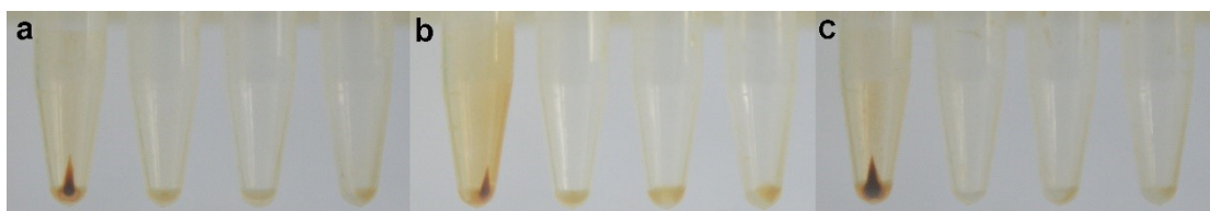
Figure S4 The photographs of precipitates in the plastic centrifuge tubes after centrifuging aqueous solution of Fol (1.6 mM, 0.5 ml) upon the addition of equivalent volume of (a) KCl, (b) NaCl, or (c) CH 3 COONa (from left to right c_{\text{Fol}}:c_{M^+} = 1:1000 , 1:500, 1:250, and 1:100). c is the molarity of alkali metal ion or Fol .
