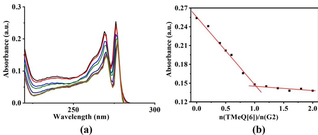
**Figure S3.** (a) The UV-Vis spectrogram of adding TMeQ[6] (0, 0.2, 0.4,...1.6, 1.8, 2.0, equivalent) to the guest G2 ( $1 \times 10^{-3}$  mol L<sup>-1</sup>, pH=2). (b) Plots of  $n(\text{TMeQ}[6])/n(\text{G}2)$  vs ultraviolet absorption of G2.
