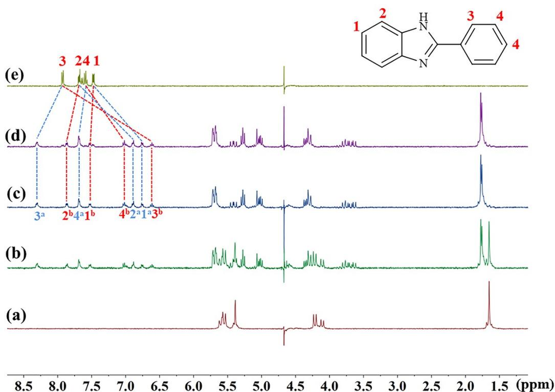
**Figure S2.** <sup>1</sup>H NMR spectra of the interaction between TMeQ[6] and G3 (25 °C, 400 MHz) (D<sub>2</sub>O, pD=2): in the presence of TMeQ[6] (0.5mM), the equivalent (a) 0, (b) 0.8, (c) 1.0, (d) 1.2, (e) pure G3
