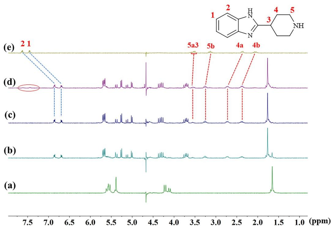
**Figure S1.**  $^1\text{H}$  NMR spectra obtained for the interaction between TMeQ[6] and G2 (25°C, 400 MHz) ( $\text{D}_2\text{O}$ ,  $\text{pD} = 2$ ): in the presence of TMeQ[6] (0.5 mM) and (a) 0, (b) 0.8, (c) 1.0, and (d) 1.1 equiv. of G2, and (e) pure G2.
