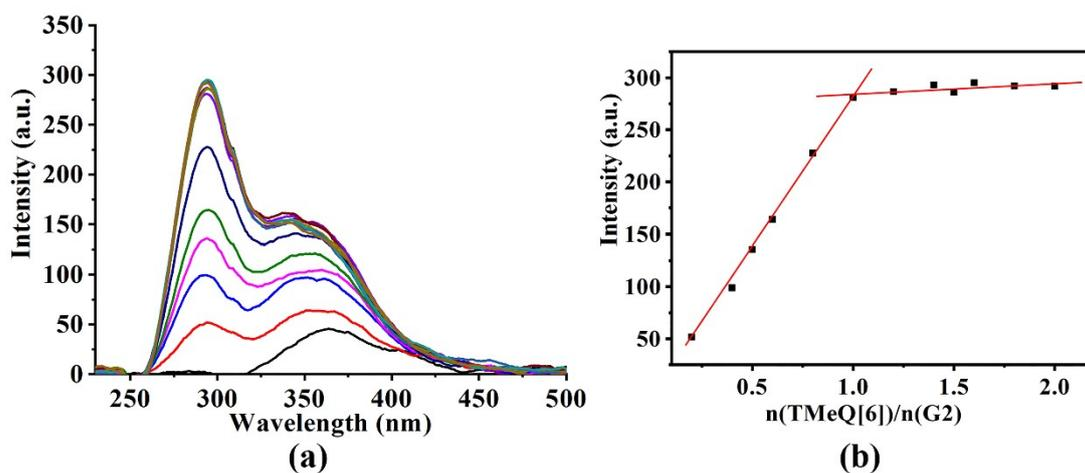
**Figure S4.** (a) The fluorescence spectra of adding TMeQ[6] (0, 0.2, 0.4,...1.6, 1.8, 2.0, equivalent) to the guest G2 ( $1 \times 10^{-3}$  mol L<sup>-1</sup>) (pH=2). (b) Plots of  $n(\text{TMeQ}[6])/n(\text{G}2)$  vs fluorescence intensity of G2.
