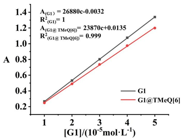
Figure S13. Calibration curves of G1 and G1@TMeQ[6].
