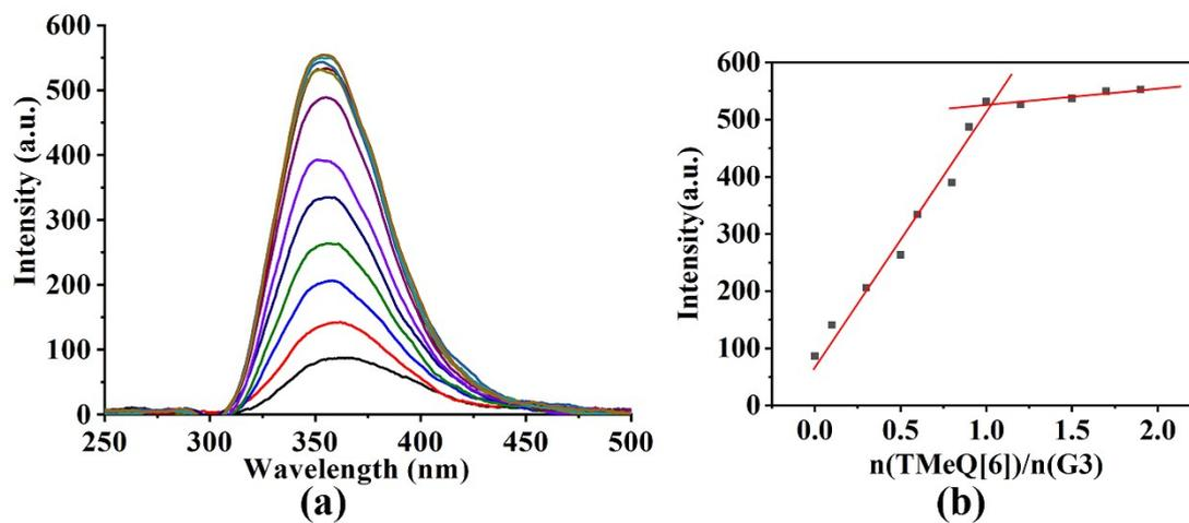
**Figure S6.** (a) The fluorescence spectra of adding TMeQ[6] (0, 0.2, 0.4, ... 1.6, 1.8, 2.0, equivalent) to the guest G3 ( $1 \times 10^{-3} \text{ mol L}^{-1}$ ) (pH=2). (b) Plots of  $n(\text{TMeQ}[6])/n(\text{G3})$  vs fluorescence intensity of G3.
