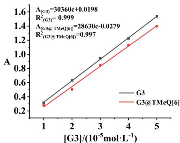
Figure S15. Calibration curves of G3 and G3@TMeQ[6].
