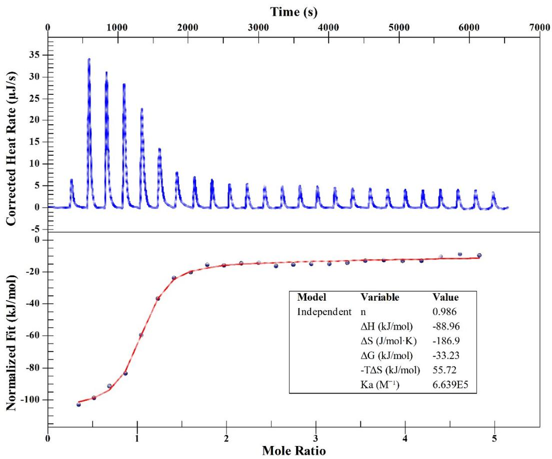
**Figure S10.** Titration diagram for isothermal titration calorimetry of G1@TMeQ[6].
