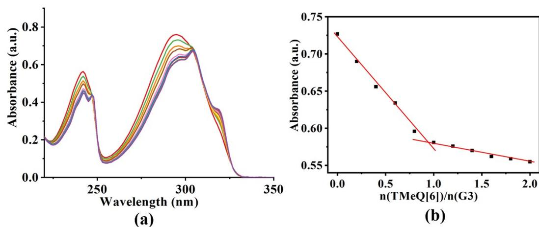
**Figure S5.** (a) The UV-Vis spectrogram of adding TMeQ[6] (0, 0.2, 0.4,...1.6, 1.8, 2.0, equivalent) to the guest G3 ( $1 \times 10^{-3}$  mol L<sup>-1</sup>, pH=2). (b) Plots of  $n(\text{TMeQ}[6])/n(\text{G}3)$  vs ultraviolet absorption of G3.
