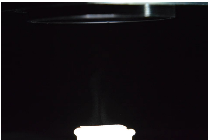
Fig. S4. Digital image showing visible steam generation enabled by the hydrophobic MXene/AuNFs membrane under 4 \text{ kW m}^{-2} illumination.
