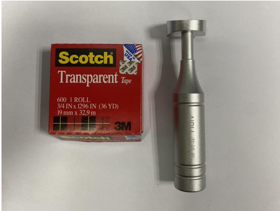
Figure S2. Peg knives for adhesion testing of adhesive tapes.
