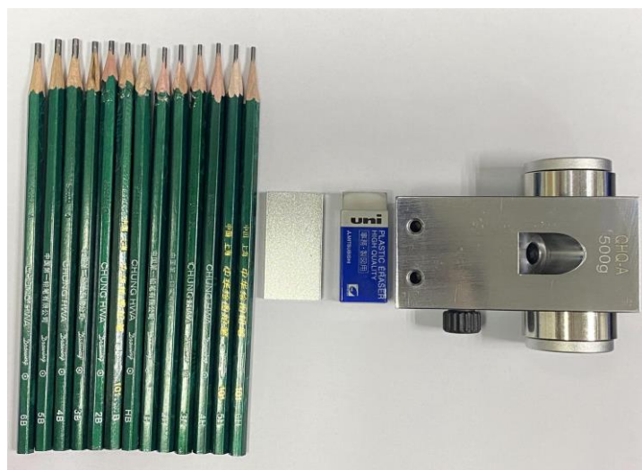
Figure S1. Pencil hardness tester for scratch hardness testing.
