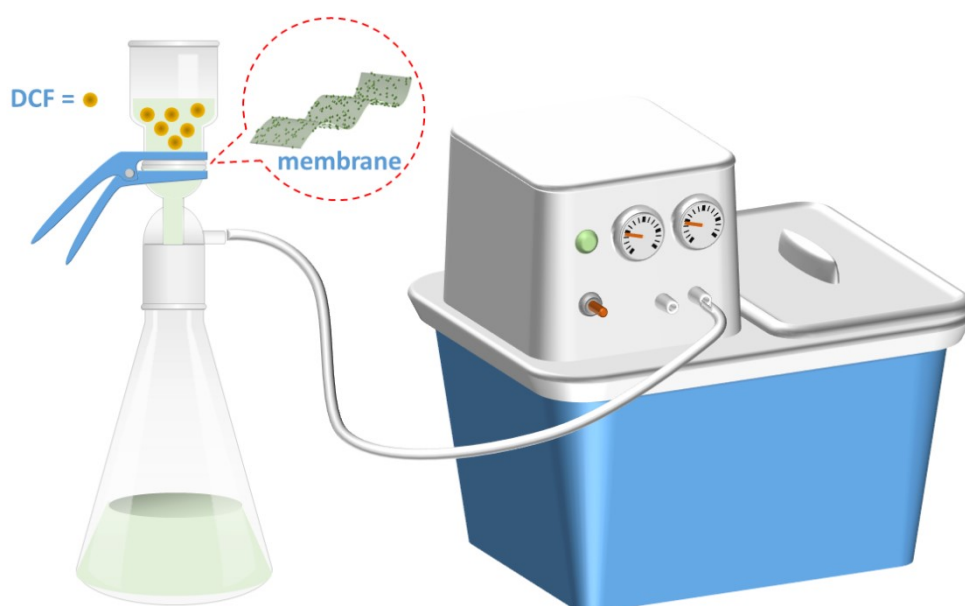
Fig S17 Schematic diagram of the experimental device for DCF removal process based on membranes.
