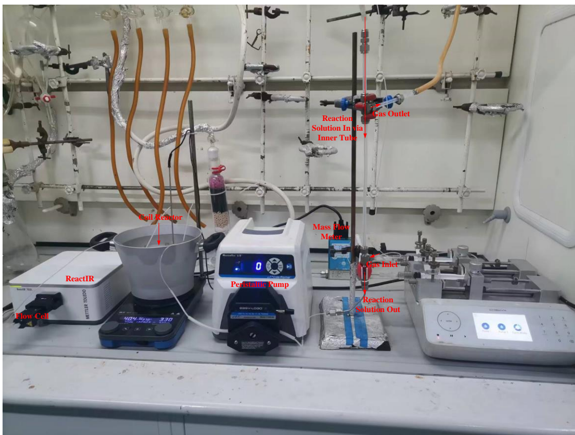
Figure S10. Photo of the experimental setup of the coaxial double-tube reactor based continuous-flow system.
