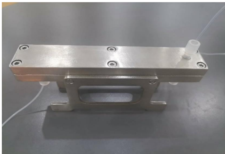
Figure S8. Photo of the liquid-liquid membrane separator.
