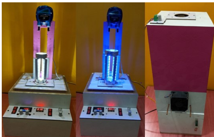
Figure 4: Falling film looping photoreactor setup equipped with different irradiation modules 1xA module (left), 2xA module (middle) and back view of the case module (right).
