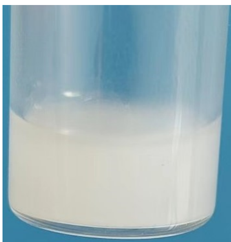
Fig. S1. The photograph of the porous liquid with 2 wt.% content of ZIF-8 in [THTDP][BTI].
