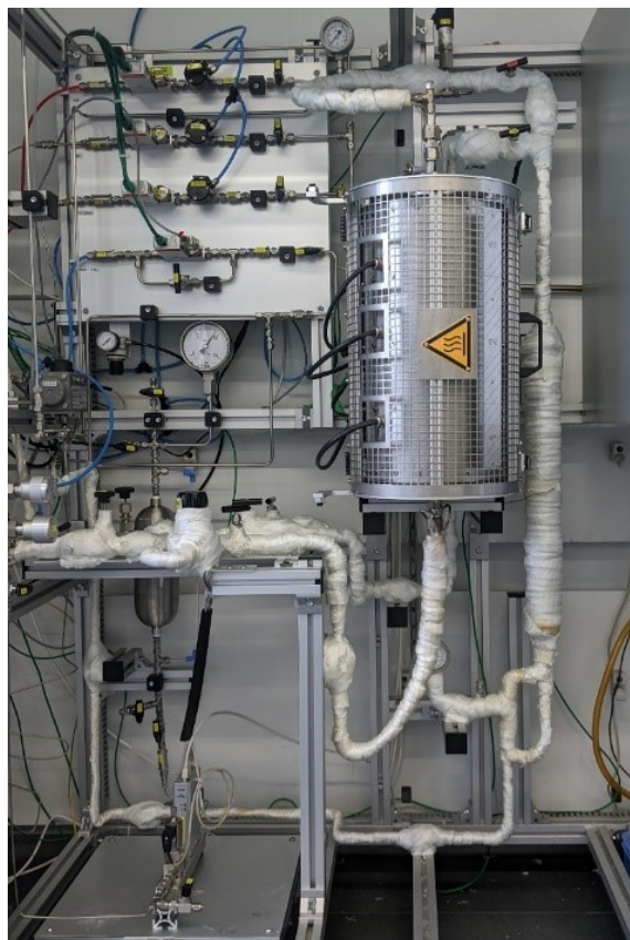
Figure S2: Image of gas-phase reactor setup used for n -heptane dehydrogenation.
