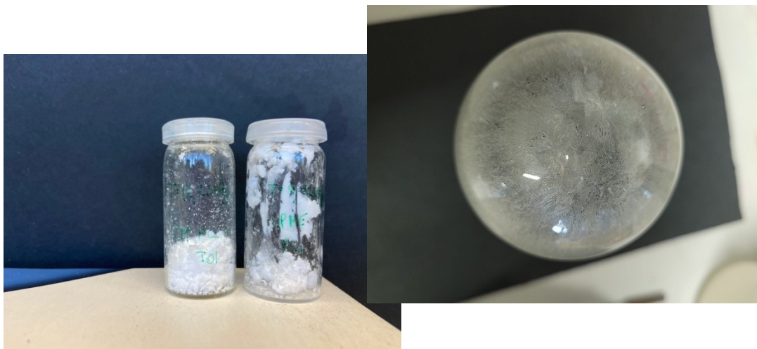
Figure S12 – Samples collected from the flow experiments starting with 2M of caprolactone (left) and with 0.17 M of caprolactone (right).
