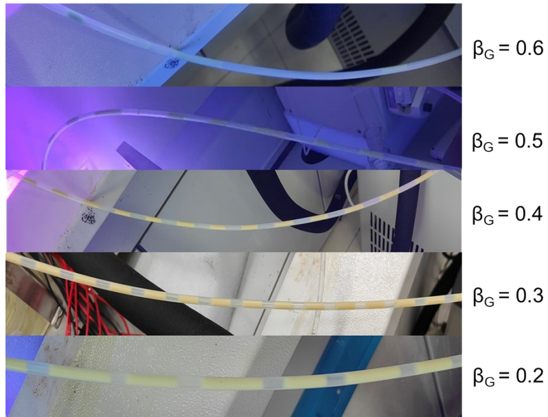
Fig. S12. Effect of gas fraction on the homogeneity and stability of slurry Taylor flow.
