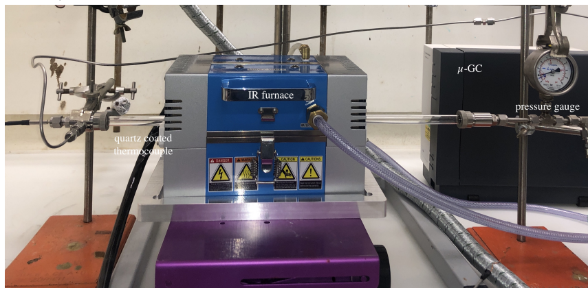
(b) Picture of catalytic test setup with IR furnace (with water cooling), quartz glass tube (ID 9 mm), μ-GC Agilent 490 and quartz coated thermocouple.
