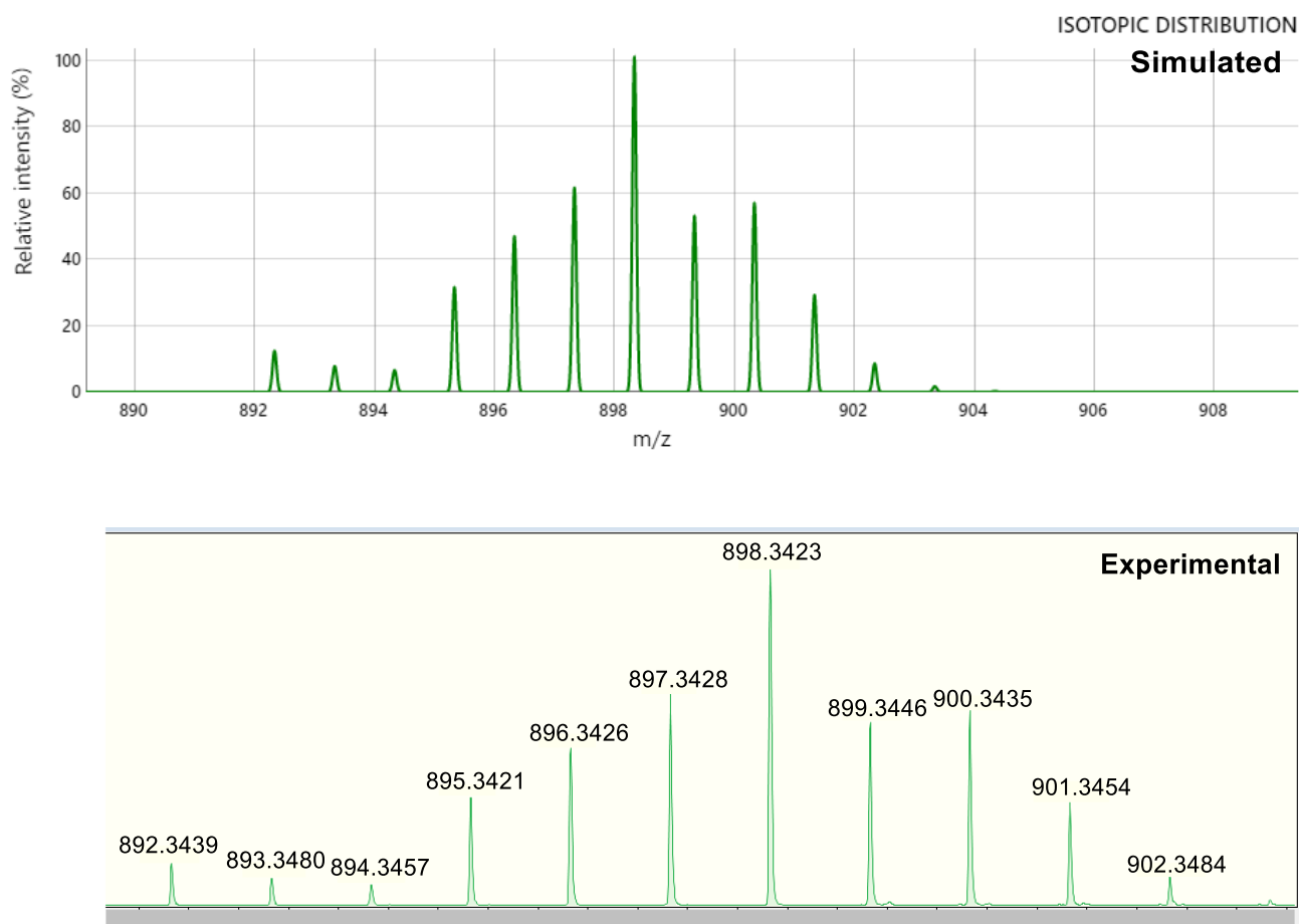
Fig. S14 HR-ESI-MS spectra showing the experimental and simulated isotope patterns of 3c .
