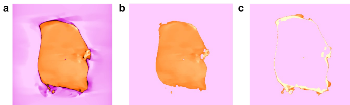
Figure S24. a. Cross section of the 1:3 blend particle, b. Inner structure/phase after separation/thresholding and c. Outer structure/phase after separation/thresholding, showing how the two phases were separated.
