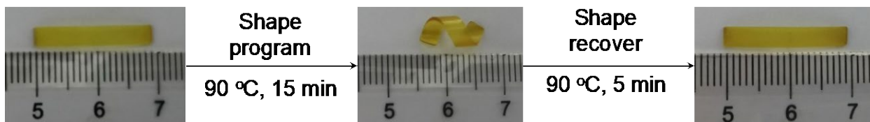
Figure S29. PUB2 film was subjected to the thermal morphing at 90 oC for 15min and then cooled for 5min while fixed. Subsequent heating at 90 °C for 5 min achieved shape recovery.
