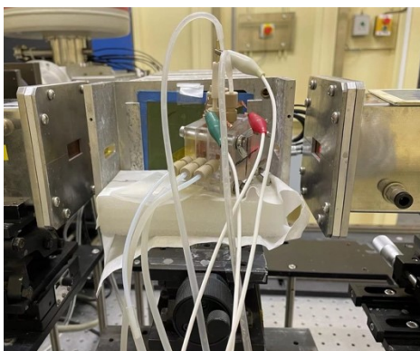
Figure S19. In situ electrochemical cell for XAS test.
