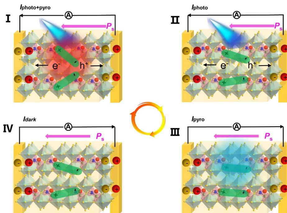
**Figure S6.** Schematic diagram for creating FPP effect with the laser being turned on/off.
