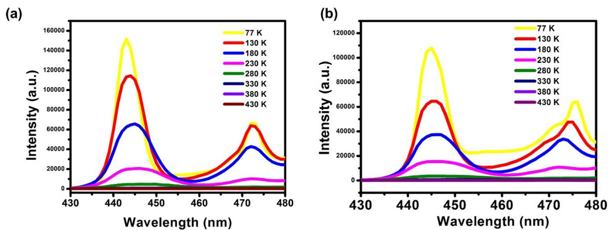
**Figure S9.** The temperature-dependent PL emission spectra of  $\text{BA}_2\text{CsPb}_2\text{Br}_7$  (a) and  $\text{BA}_2\text{Cs}_{0.66}\text{MA}_{0.34}\text{Pb}_2\text{Br}_7$  (b).
