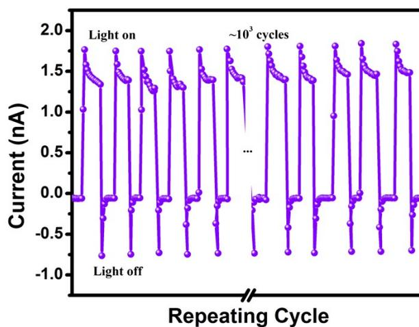
**Figure S7.** The long-term stability of the photodetector of  $\text{BA}_2\text{CS}_{0.66}\text{MA}_{0.34}\text{Pb}_2\text{Br}_7$ .
