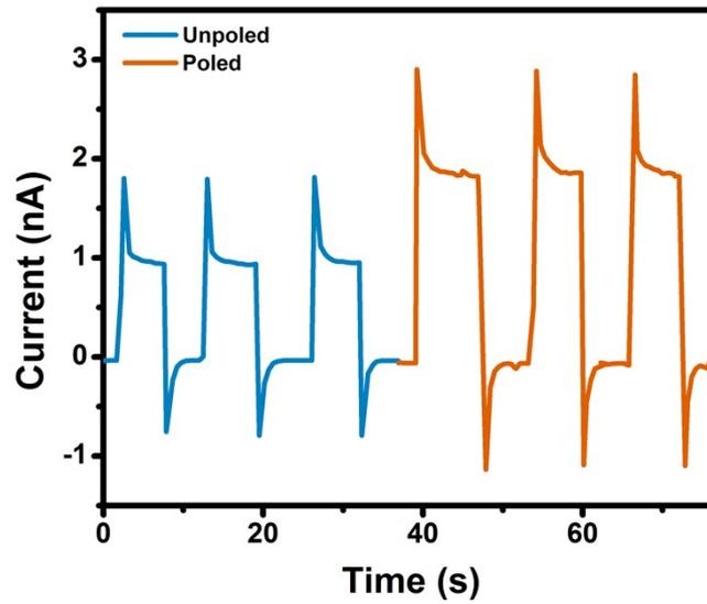
**Figure S10.** *I-t* curves of  $\text{BA}_2\text{Cs}_{0.66}\text{MA}_{0.34}\text{Pb}_2\text{Br}_7$  before and after device electric field polarization.
