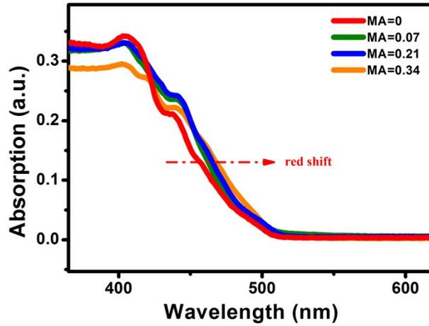
**Figure S3.** UV-vis absorption spectra of  $\text{BA}_2\text{Cs}_{1-x}\text{MA}_x\text{Pb}_2\text{Br}_7$  ( $x = 0, 0.07, 0.21, 0.34$ ).
