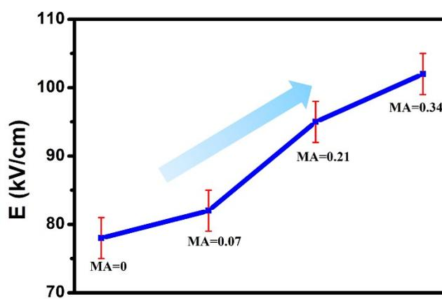
**Figure S2.** The breakdown resistance voltage of  $\text{BA}_2\text{Cs}_{1-x}\text{MA}_x\text{Pb}_2\text{Br}_7$  (x = 0, 0.07, 0.21, 0.34).
