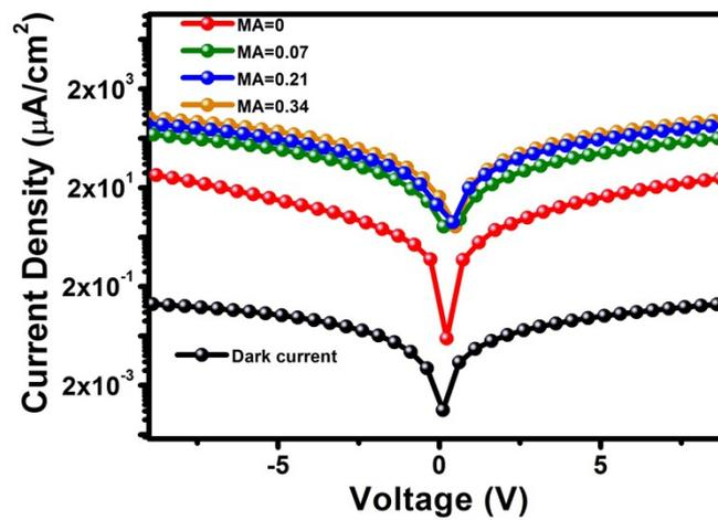
**Figure S4.** The photo-electric characteristics of mixed cage cation samples under 405 nm laser irradiation (10 V, 74 mW/cm<sup>2</sup>).
