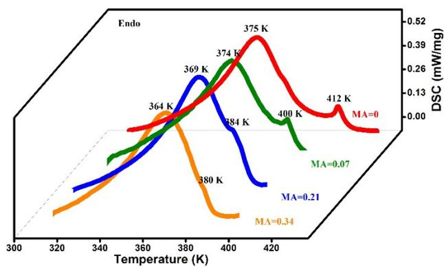
**Figure S1.** DSC curves of  $\text{BA}_2\text{Cs}_{1-x}\text{MA}_x\text{Pb}_2\text{Br}_7$  (x = 0, 0.07, 0.21, 0.34).
