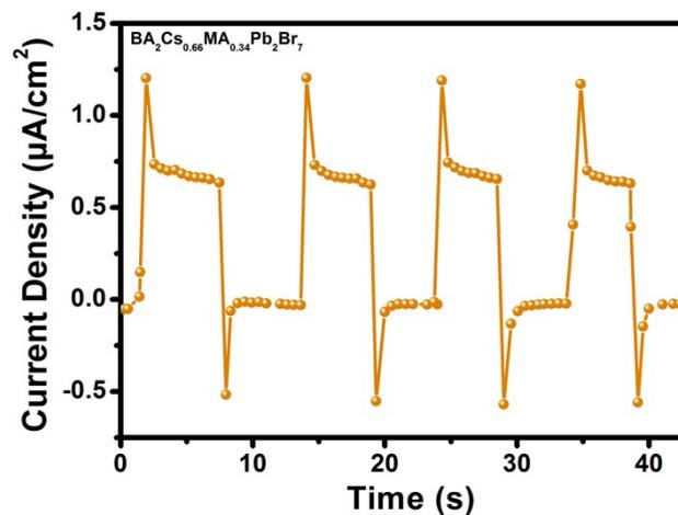
**Figure S5**  $I-t$  curves under 450nm light illumination.
