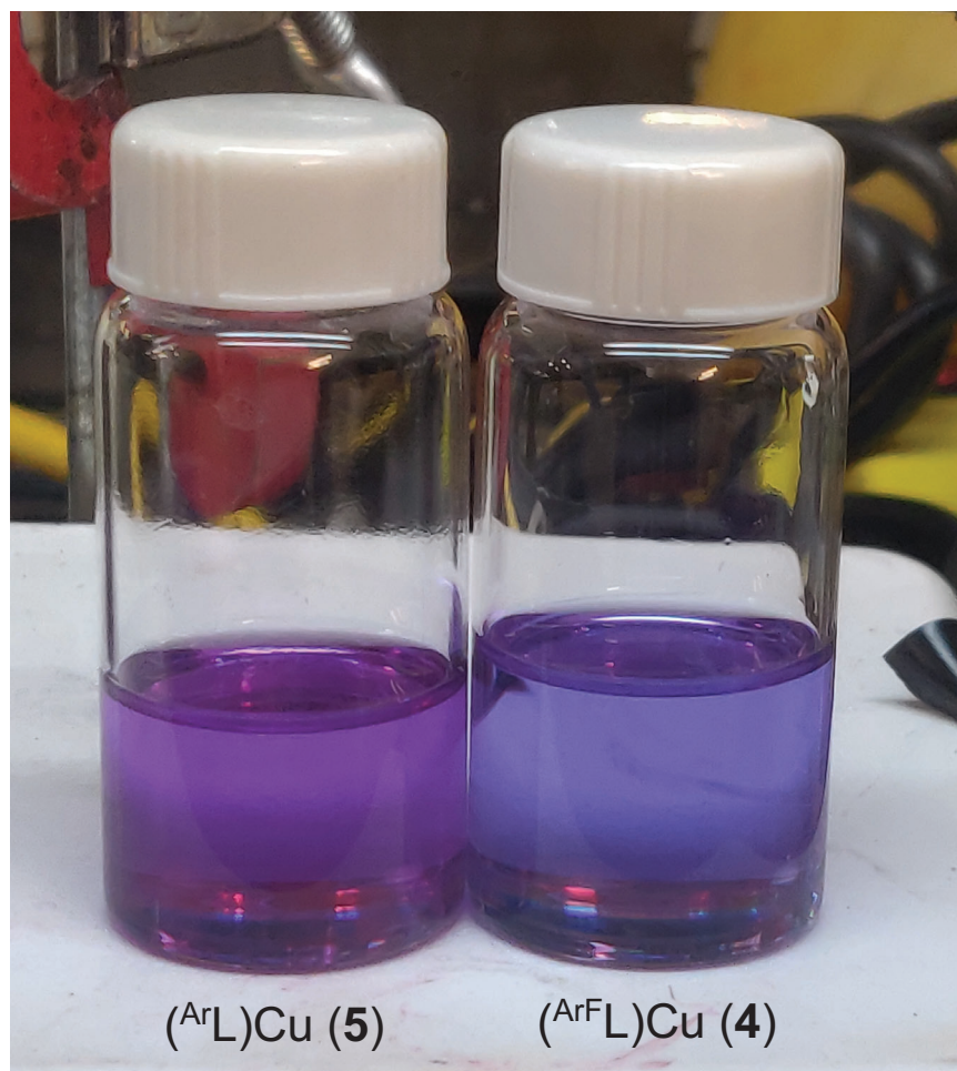
Figure S78. Visual comparison of (^{Ar^F}L)Cu (4) ( right ) and (^{Ar}L)Cu (5), displaying a visible shift in apparent color as a function of meso arene fluorination. Both solutions are 20 \mu M concentration in benzene.
